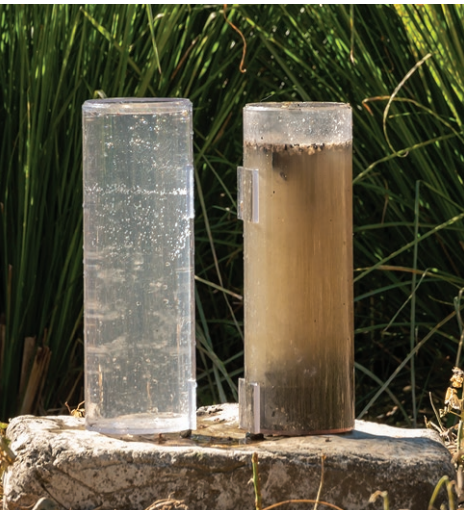
Water quality samples demonstrate the clarity of water before (right) and after (left) filtration in TNC's artificial marshes in Jarabacoa, Dominican Republic © Ricardo Briones
