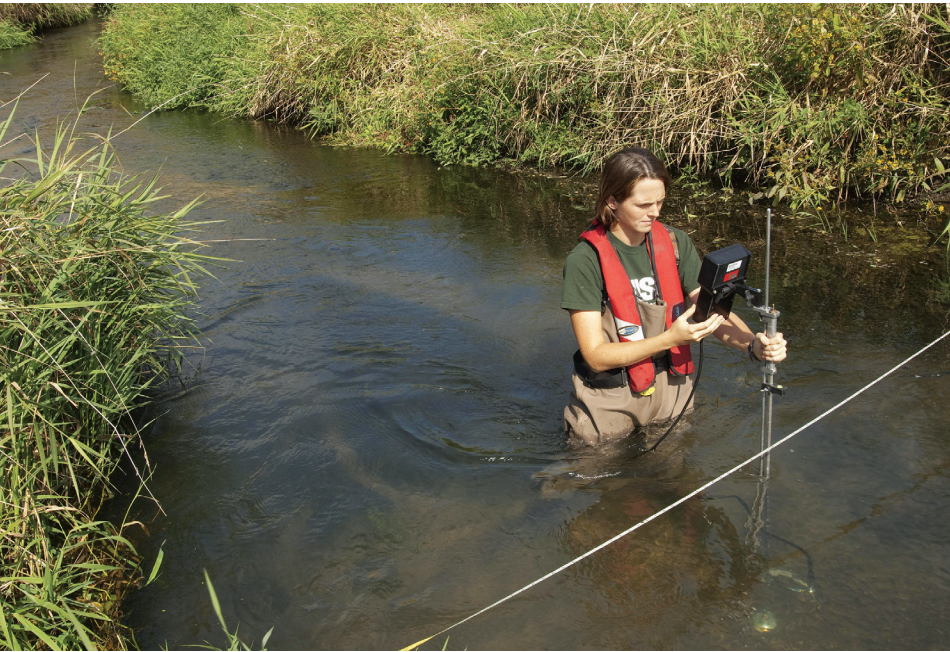
Researcher determines water volume flowing through a recently restored stream © Mark Godfrey/TNC
