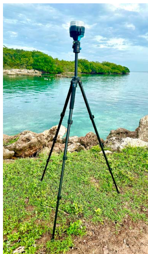
Figure 24. A GNSS base station collecting position correction data during a UAS mission
