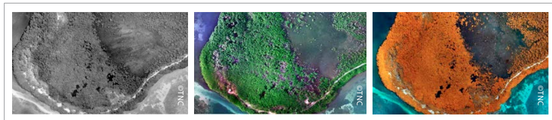
Figure 11. Three types of aerial photography (left to right: panchromatic ; natural colour ; and colour infrared )
