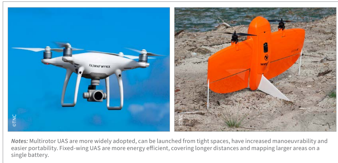
Figure 23. Examples of a multirotor (left) and a fixed-wing (right) UAS
