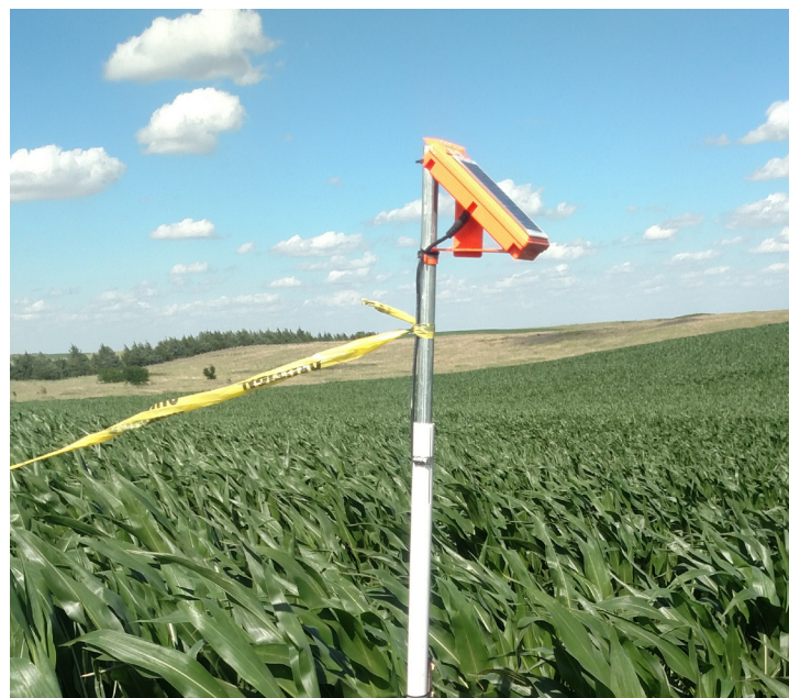
A solar-powered communication tower sends soil moisture levels to both farmers and researchers © Patrick Janssen
